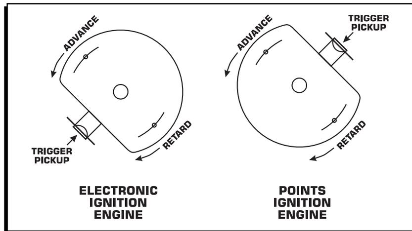
**Figure 14 Adjusting the Timing on a Tecumseh**
