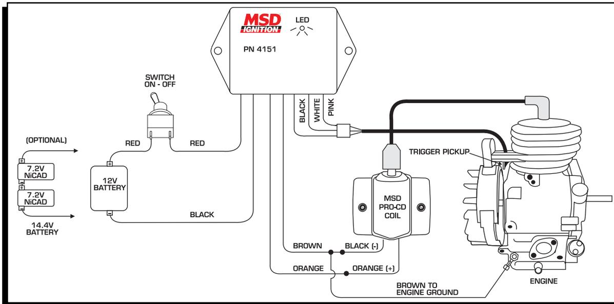
**Figure 11 Wiring the MSD Ignition System.**
