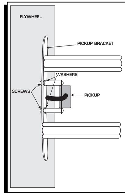
**Figure 7 Adjusting the Airgap.**
