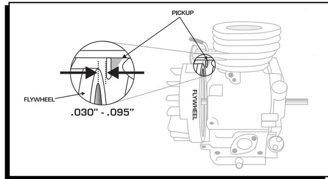
**Figure 6 Checking the Air Gap of the Flywheel and Trigger Pickup.**
