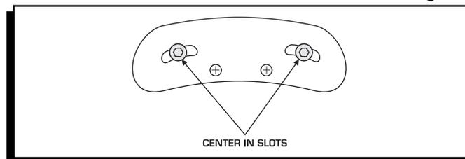
**Figure 8 Positioning the Pickup Assembly of a Briggs & Stratton Engine.**
