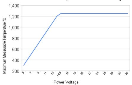
Maximum Measurable Temperature vs Power Voltage
