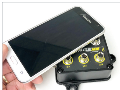
5. TOUCH and HOLD the mobile device on the CL1 data box.
