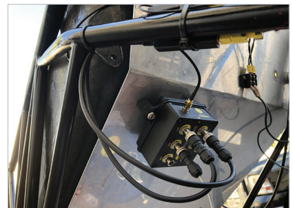
6. Racepak suggests mounting the CL1 on the rear cockpit firewall, in an easily accessible location.
