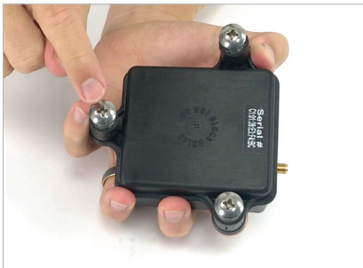
4. The CL1 Data Box can be mounted in any direction, via the three rubber isolation mounting feet.
