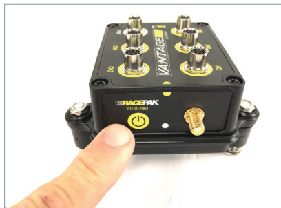
5. Ensure the Power / LED Status Indicator and sensor ports are in view and accessible.
