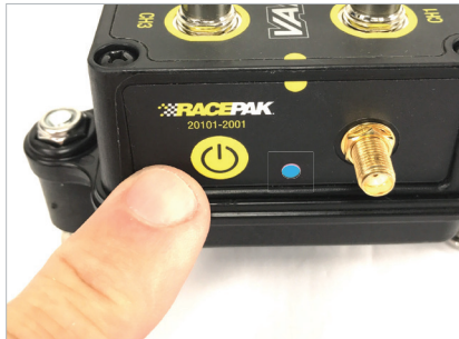
1. Briefly press the power button on the CL1 data box. The LED will turn BLUE.
