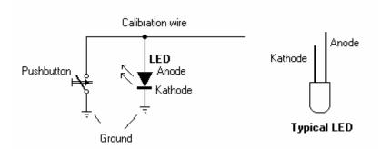
The LED will communicate the LC-1's status. To monitor LC-1 status, connect the red wire (Anode) of the included LED to the calibration wire (black) of the LC-1 and connect the black wire (Cathode) of the LED to the ground wire of the momentary switch. The grounds to both the cathode side of the LED and the Push button should be connected with the Heater ground.
