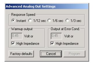
When setting the LC-1 to the slower response speed settings the measured mixture data will be averaged over the response time setting before being output.
