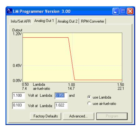
This shows the analog output voltages versus Lambda for one of the two analog outputs. The graph display is automatically scaled to the selected voltages. For each output you can specify a minimum and maximum lambda value and the associated voltages. Below the minimum and above the maximum lambda values the output voltages stay constant at the associated programmed voltage.
