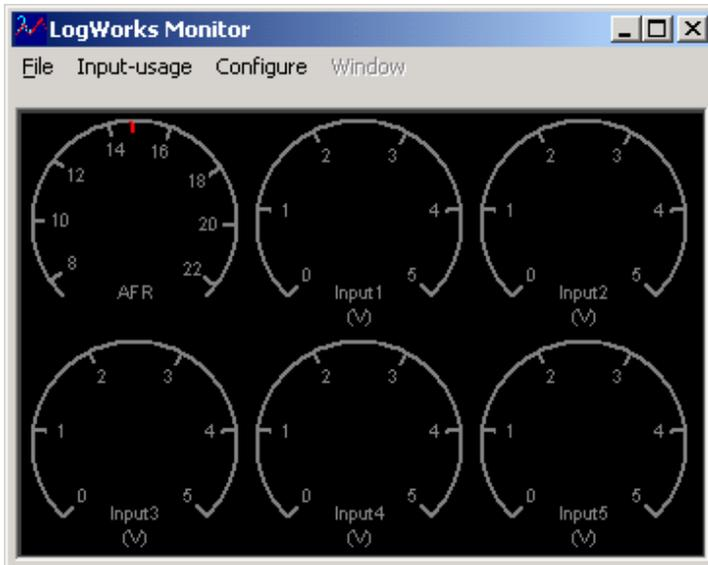
This window is resizable by grabbing on the lower edge of the window. The round gauges are typically arranged in a 3 x 2 arrangement. This arrangement will be changed depending on the window width and height to maximize the gauge size. All gauges are greyed out until:
