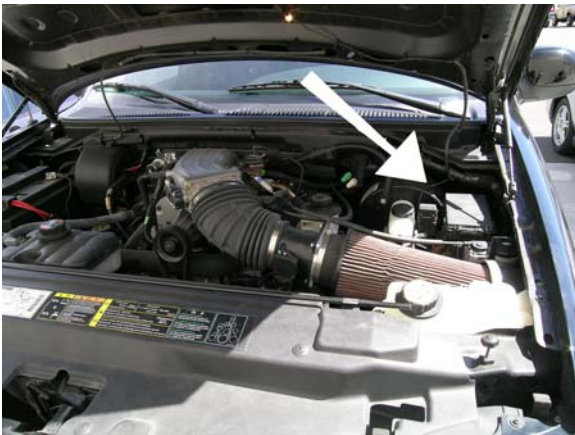
This is the location of the fuse box (under the hood on the right side)
