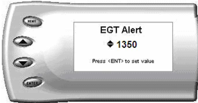
4. Press the up and down arrow keys until you see the desired EGT level at which you want to be alerted and press [Enter] to set that value.
