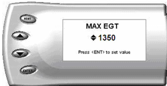
2. Change the Max EGT set point by pressing the up and down arrow keys to select the maximum temperature that you want the exhaust gas temperature to reach, then pressing [Enter]. When the exhaust gas temperature reaches this value, the power delivery will be decreased to prevent the temperature from exceeding this set value.
