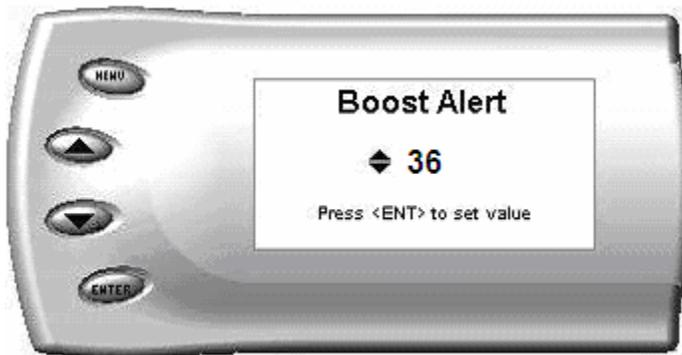
6. Press the up and down arrow keys until you see the desired Boost level at which you want to be alerted and press [Enter] to set that value.
