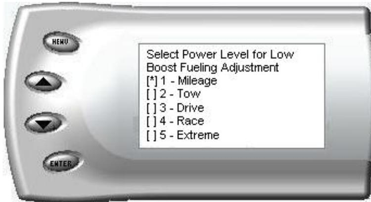
Select the power level for which you want to adjust the low boost fueling and press Enter. When you press Enter, the following screen appears allowing you to select the Low Boost Fueling Adjustment level that will be unique to that level and every time you select that power level the fueling adjustment will be set to what you chose on this screen.
