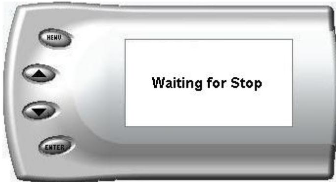
4. When your vehicle is at a complete stop, the following screen automatically appears:
