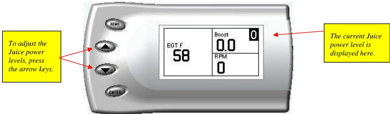
**NOTE:** The 3 stage power switch on the Juice module is disabled when the Attitude monitor is installed. (The switch does not have to be set at a certain power level when the Attitude module is installed.) Power levels must be adjusted using the Attitude module.
