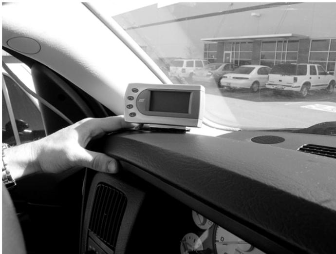
*After the bracket is mounted, use the supplied two-sided tape to secure the Attitude to the bracket.*
