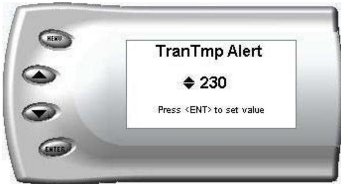
10. Press the up and down arrow keys until you see the desired Transmission Temp level at which you want to be alerted and press [Enter] to set that value.
