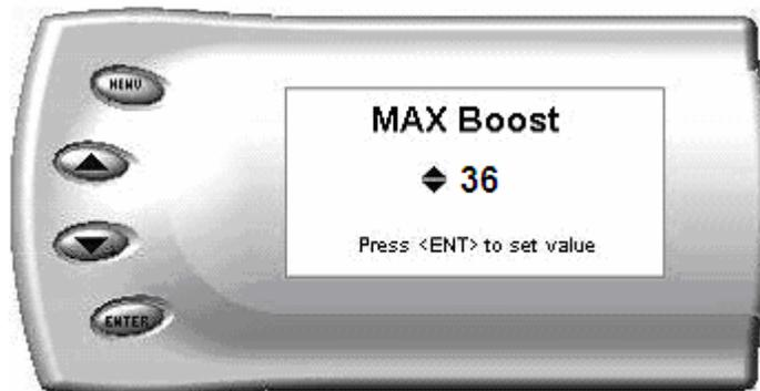
3. Change the Max Boost set point by pressing the up and down arrow keys to select the maximum pounds of boost that the turbo is allowed to produce. Once the number is set, press [Enter]. When the boost level reaches this value, the power delivery will be reduced so as not to allow the boost to exceed this set value.
