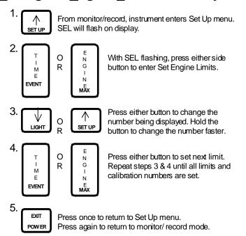
Function limits are set in the following order: Delay Time, Temp (C1), Temp(C2), Temp(C3), Water Temperature, Tach (RPM1), Tach calibration number, JS(RPM2), and JS calibration number (minus any functions that you do not have). Also, if you are not using any functions on your instrument, set its limit to any number greater than 200.
