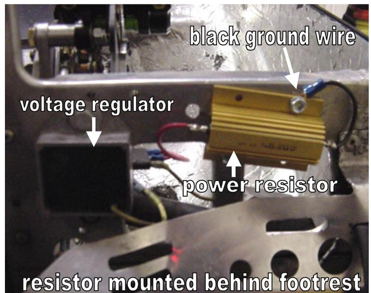
3. Connect the red wire to the lighting coil voltage (usually a heavy yellow wire). If mounting near the front of the sled on a Polaris, the red wire from the resistor can be plugged into the yellow wire on the wiring harness connector. If mounted near the voltage regulator, the red wire can be connected (spliced) to the yellow wire from the voltage regulator. Be sure this is a good solid connection.
