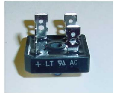
rectifier markings on the side
