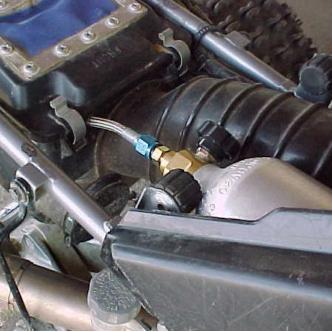
The nitrous manifold, solenoid, and rectifier are shown above.
