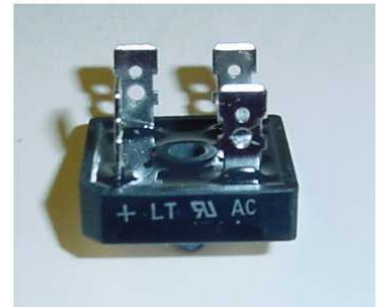
rectifier markings on the side
