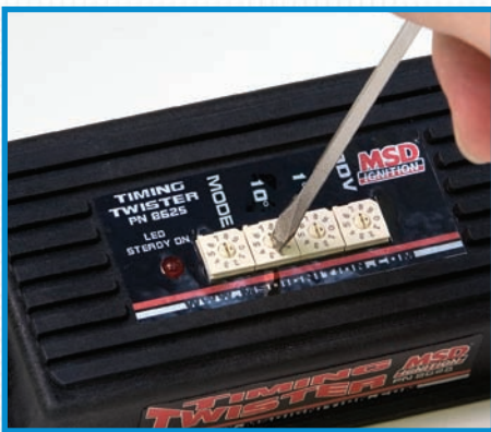
Adjustments to the timing are easily made with a twist of a rotary dial.
