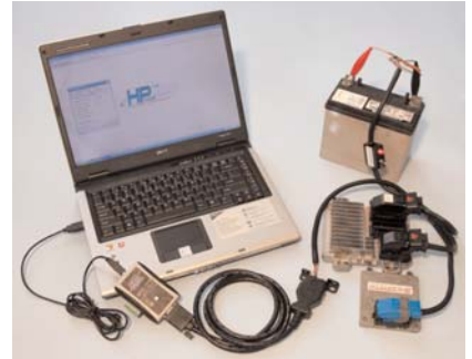
Custom tuning modern controllers typically requires software and a connection harness. The photo shows the typical out-of-car setup for flashing an E67 ECM and T42 TCM through a Speartech harness ($185) and HP Tuners interface ($499).
