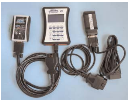
Communicating, reading, and re-flashing late-model flash-based controllers can be done using the appropriate interface module. Several tuning options exist allowing users to shop for an interface that suits their needs and budget. Three Gen IV systems GMHTP has tested include HP Tuners ($499), EFI Live ($749), and LS2-Edit ($550), as shown from left to right.
