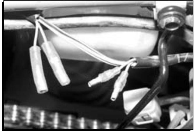
Figure 5 Installing the Bullet Connectors to the Pickup Wires.
