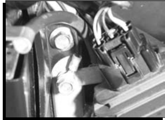
Figure 9 Connecting the Main MSD Negative wire.
