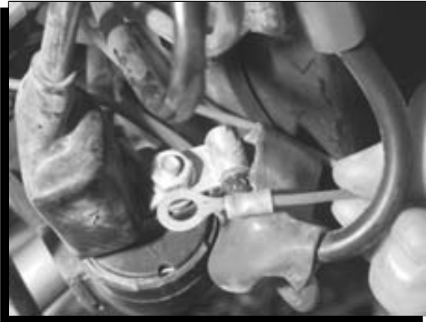
Figure 8 Connecting the Main MSD Positive Wire.
