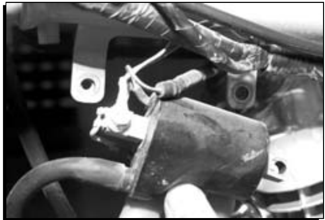
Figure 6 Removing the Original Coil.
