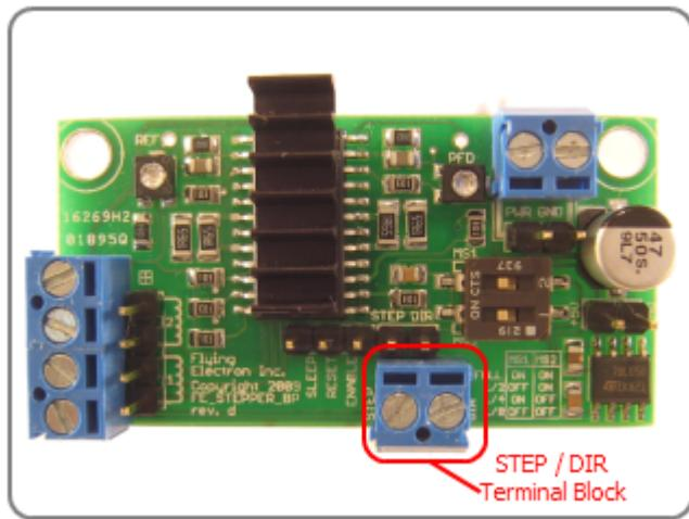
Important! The equipment connected to the Step and Dir signals must share a common ground with the driver board. If in doubt, the ground of the equipment supplying the Step and Dir signals should also be connected to the GND terminal block. If the Step and Dir signals appear to work erratically or not at all, make sure there is a common ground shared by the source of the Step and Dir signals and the driver board.
