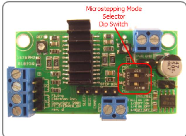
The microstepping mode is adjusted through the MS1 and MS2 dipswitches. The dipswitch has a label "ON" to signify which position of the dipswitch is the "ON" position. The "ON" position is towards the left side of the board, MS1 is towards the top of the board, and MS2 is towards the bottom of the board. The settings are as follows:
