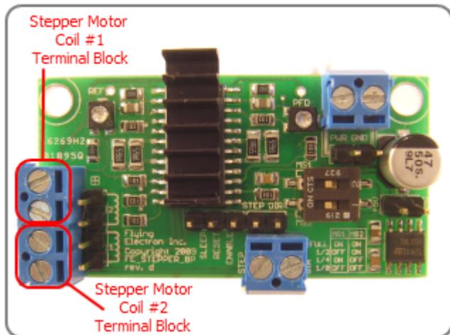
**Important!** After connecting the wires to the terminal blocks, gently pull on the wires to make sure they are securely attached to the terminal blocks. A loose wire or bad connection will cause permanent damage to the drive board.
